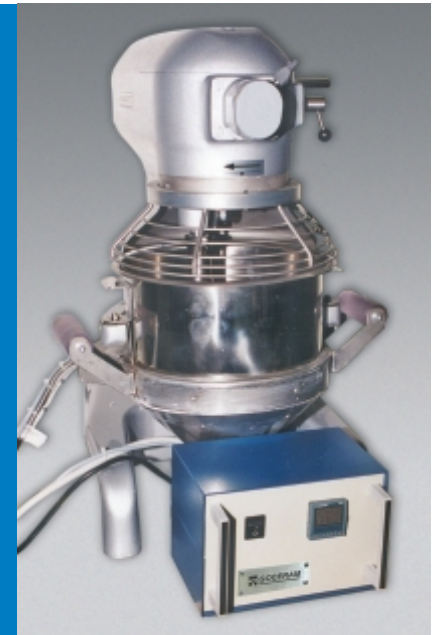
Feedstock mixer, 5 litre, with heat unit
